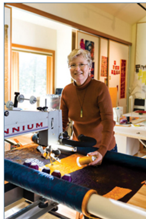
EASY REACH: The long arm of the quilting machine is 24 inches—so the area in which a quilter can work feels relatively vast.
